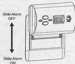
2. Place mounting plate in desired location and install two screws provided. Tighten screws until mounting plate is secure. Do not overtighten screws as damage could occur. If mounting into plasterboard or drywall, drill a 3/16" hole in the wall and use the two plastic anchors provided.
